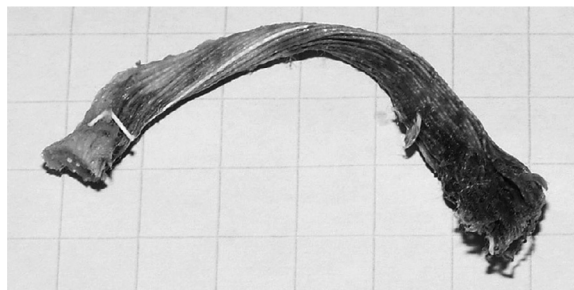
Figure 7.17 The Stryker ® ligament is made of multilayers of polyethylene terephthalate (PET) and polyester (Dacron ® ).
